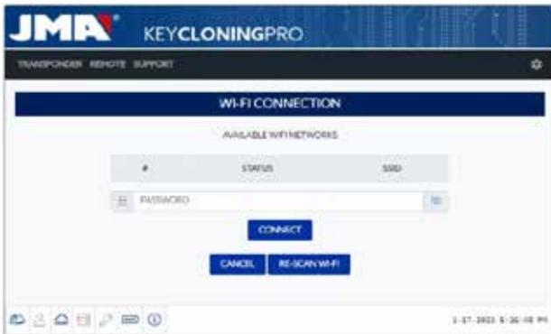
From this page (after pressing RE\_SCAN WI-FI), scan all the Wi-Fi networks within range of the EvoXpert (hidden Wi-Fi networks cannot be configured).
