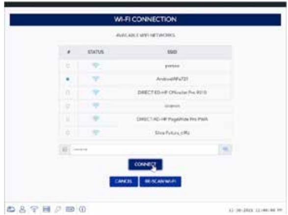
After pressing **CONNECT** and waiting for your EvoXpert to restart (the Status LED completes the Green-Red-Green cycle), you will have configured the Wi-Fi connection on your EvoXpert to work with the Hotspot Wi-Fi network on your mobile.
