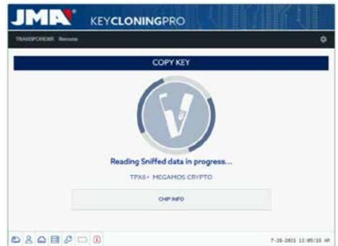
If the operating mode change process continues correctly, the following menu will be displayed telling you to collect data from the vehicle ignition lock.
