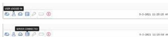
After completing the three steps above (and in the EvoXpert example used), you should see the first four icons on the lower toolbar activated. Pressing the Tools icon (on the right, in the upper Menu bar) will open a drop-down menu. If you select the CONNECTIONS option, you will be shown the communication parameters explained in Section 4 in more detail.
