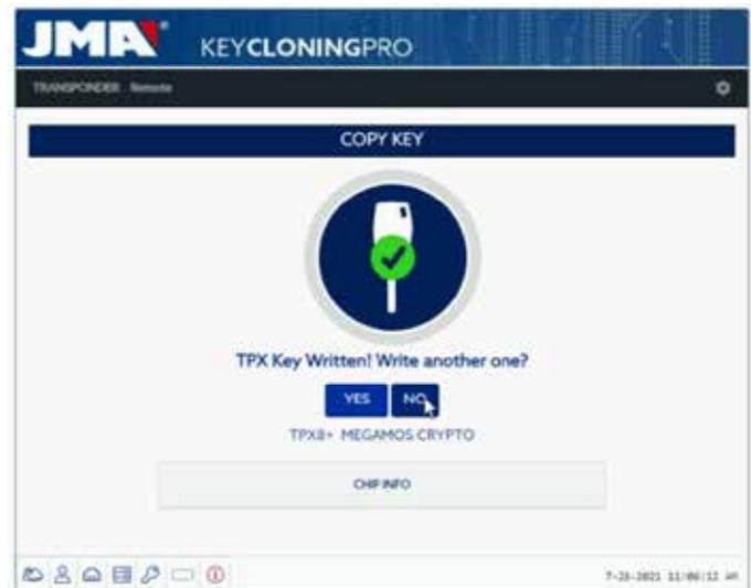
If you do not wish to make another copy right now, press NO so that the key is deleted from both the Pending Keys process on the server and the task control panel on the client machine.
