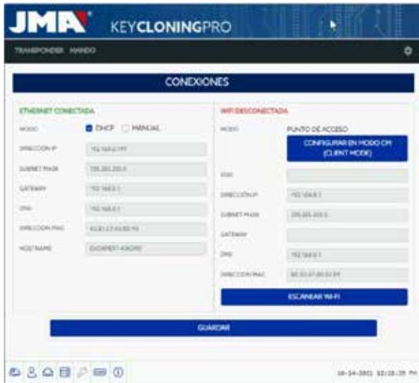
Once this page is open, you can change the Wi-Fi configuration on your EvoXpert (which comes in AP Mode by default) by pressing Wi-Fi SCAN. This will refresh the WI-FI CONNECTION page.
