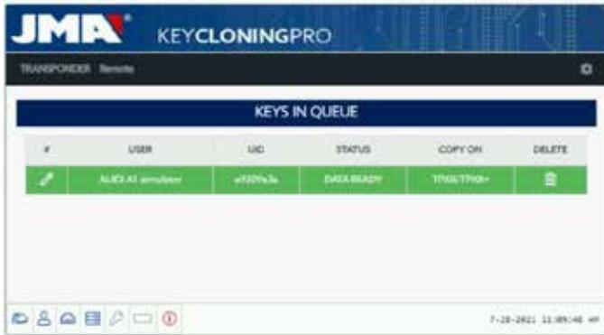
Having reached this stage of the process and the server has the code for your key ready, there are two ways to proceed with the final copy onto the blank JMA transponder indicated in the panel under the Copy to TPX8/TPX8+ column.
