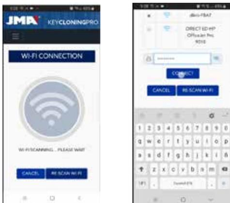
After entering the Wi-Fi network settings, after pressing CONNECT and while waiting for your EvoXpert machine to automatically restart itself, you can connect the display device (the mobile in this case) to the same Wi-Fi network because all the devices (EvoXpert and connection device being used as a display) must be on the same network.
