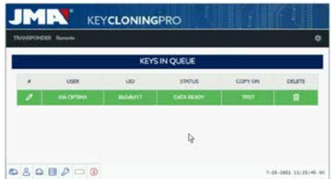
As is the case with the Megamos key we used in the previous example, there are two ways to proceed with the final copy onto the blank JMA transponder indicated under the "Copy On" column: TPX7.
