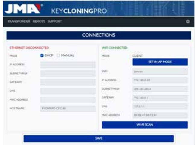
Once the EvoXpert is connected via Wi-Fi to the client router, you just need to connect the device you will be using as your display (mobile/tablet/PC/laptop) to the same Wi-Fi network on the client router. This is because both the EvoXpert machine and the display device you want to use (mobile/tablet/laptop) must be connected to the same network. Once they are both connected to the same network, you will be able to use your EvoXpert from any web browser.
