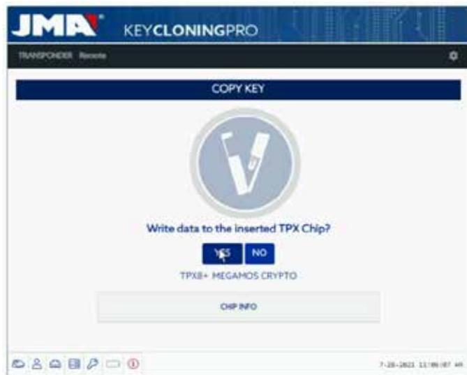
2. If you have several different keys in the panel with different technologies (Megamos, Philips, Texas, etc.), you will need to select the key you want to copy (click on the pencil icon in the first column of each row of keys that have previously reached the "Key Found" status (green), which clearly indicates that the data are ready on the server and that they need to be sent to the JMA TPX chip indicated under the COPY ON column:
