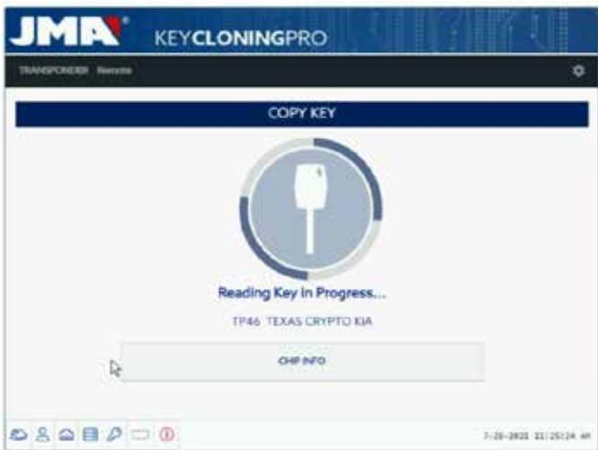
In this case, we can see the scan from a KIA Optima with key technology based on Texas DST80 and the DST80-FAST, based on the calculation time required on the JMA servers.
